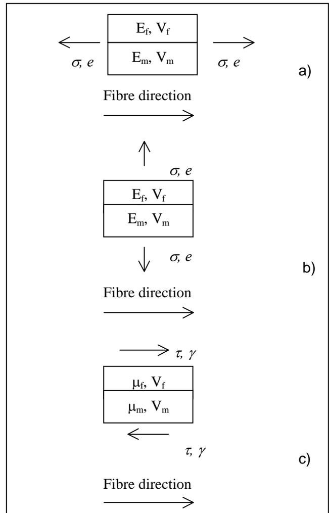
Figure 1. Deformations of a simple model of a composite material; a) axial extension, b) transverse extension, c) axial shear
