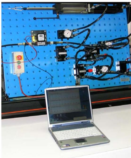
*Figure 2: Laboratory hydraulic installation with equipment for particle contamination monitoring*
