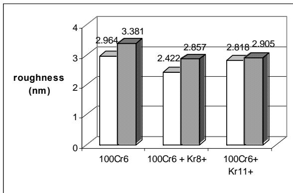
Figure 3: AFM surface roughness – 100Cr 6 steel
