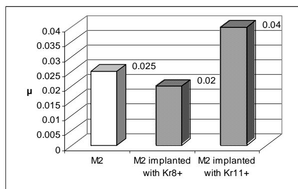
Figure 6: Friction coefficient  $\mu$  - steel M2,  $F=10N$ .
