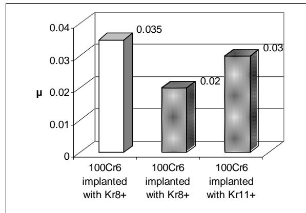
Figure 5: Friction coefficient  $\mu$  - steel 100Cr 6,  $F=10N$ .
