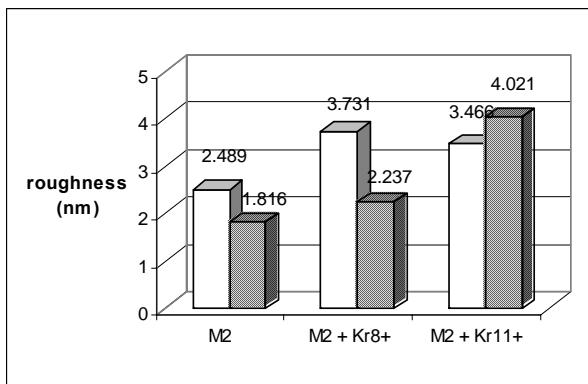
Figure 4: AFM surface roughness – M2 steel
