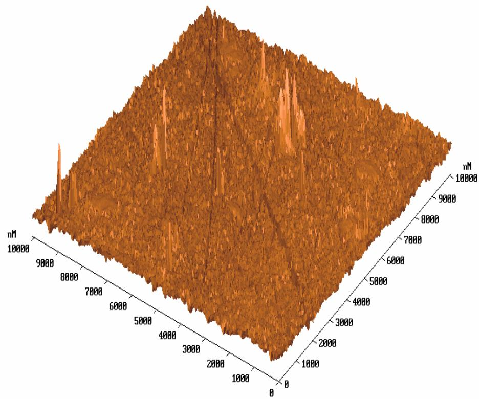
Figure 7: AFM image of surface roughness – M2 steel after Kr 8<sup>+</sup> implantation.
