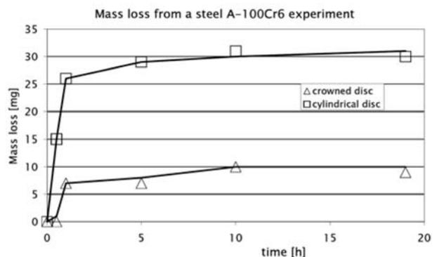
**Fig. 9:** Typical mass loss over time chart. The running in period (first hour) is clearly seen
