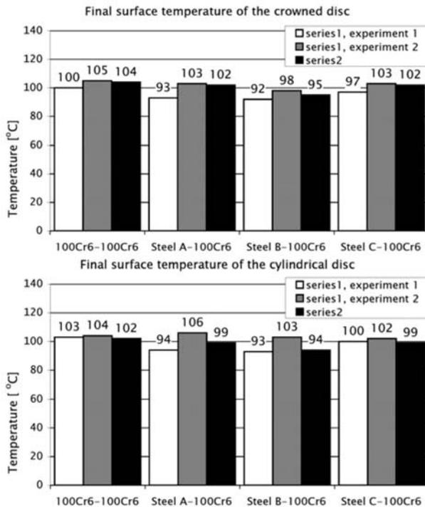
Fig. 13: Final surface temperature near the contact area
