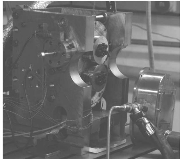
**Fig. 1: The two-disc test rig with parallel shafts of the Laboratory of Machine Elements and Machine Design**
