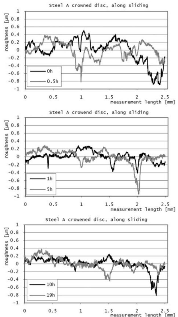
Fig. 12: Surface roughness of a steel A disc, along the sliding speed
