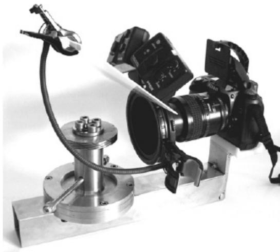
**Fig. 3: The custom-made device for circumferential photographing of the discs**
