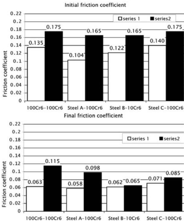
Fig. 10: Initial and final friction coefficient
