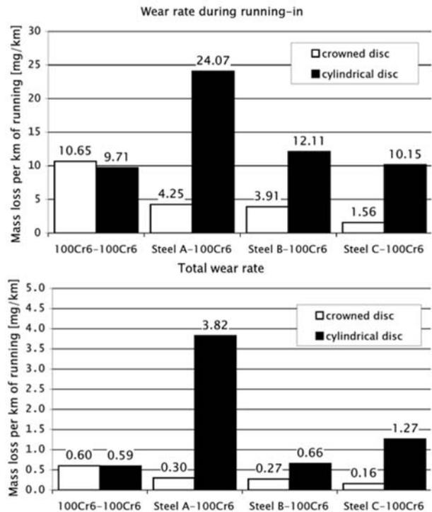
**Fig. 8:** Wear rate during running in and total wear rate. The wear rate was obtained by reducing the mass loss to the length of sliding
