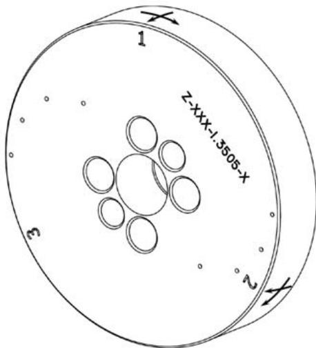
**Fig. 4: Illustration of a test discs with the three predefined points of roughness measurements marked. The two different directions (along and across sliding speed) are marked with arrows**
