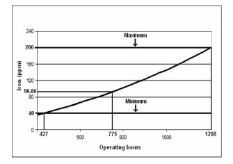
Fig.7: Extrapolation analysis result and limit values of Iron (Fe)
