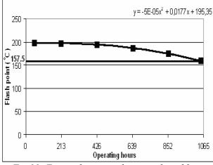
Fig.11: Extrapolation analysis result and limit value of Flash Point
