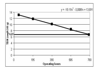
Fig.8: Extrapolation analysis result and limit value of Total Base Number (TBN)
