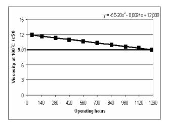
Fig.10: Extrapolation analysis result and limit value of Viscosity (100°C)
