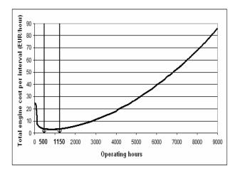
*Fig.4: Total engine cost per interval and operating hours profile*
