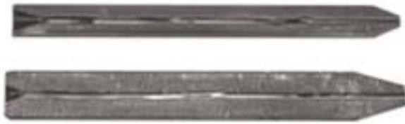
**Figure 5.** Characteristic appearance of focusing tube wear
