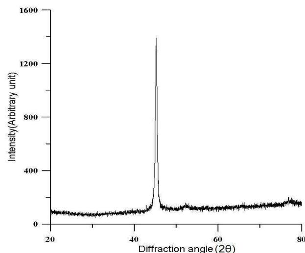
**Fig. 6.** XRD plot of as deposited coating.
