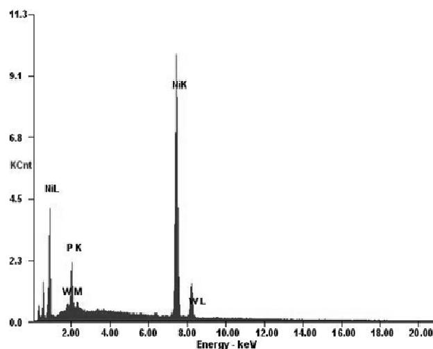
**Fig. 4.** EDX spectra of coated surface.
