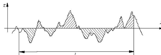
**Fig. 1.** Rough surface with a sampling length L.
