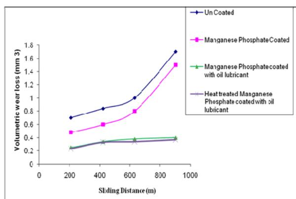
**Fig. 1.** Volumetric wear loss vs sliding distance at velocity of 3.0 m/s.
