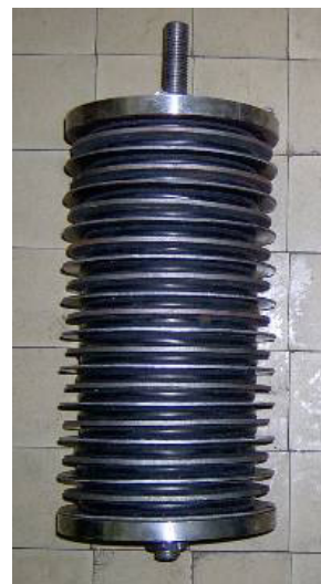
Fig. 1. Rubber-metal spring assembly of buffing gear.
