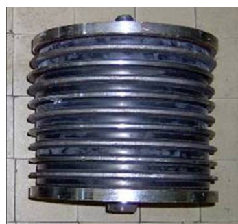
Fig. 2. Rubber-metal spring assembly of draw gear.
