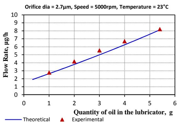
**Fig. 11.** Variation of theoretical and experimental flow rate with quantity of oil in the reservoir.
