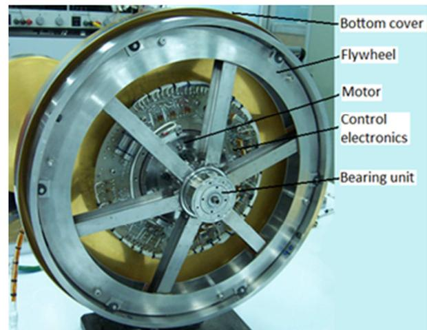
Fig. 1. Momentum wheel with top cover removed [6].
