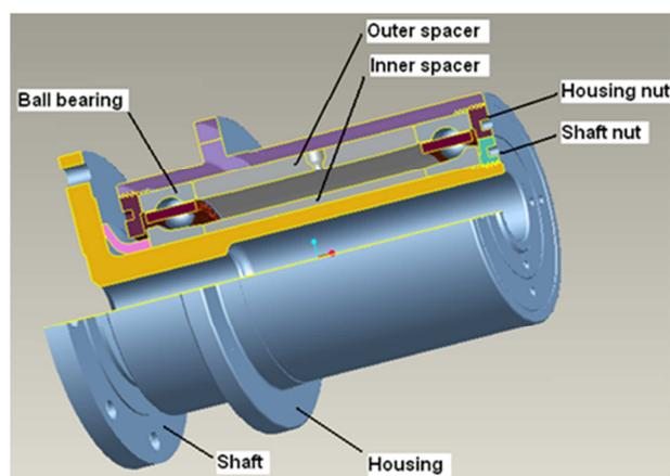
**Fig. 2.** Bearing cartridge assembly.
