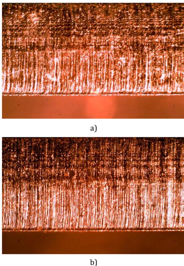
**Fig. 2.** Laser cut surface patterns obtained in trial 6 (a) and trial 27 (b).
