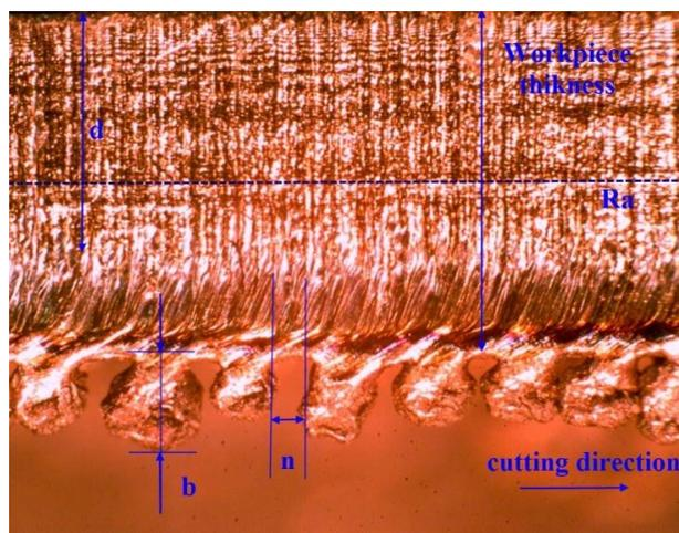
**Fig. 1.** Laser cut surface characteristics considered in the multi-criteria analysis.
