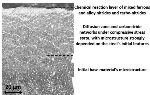
**Fig. 1.** Typical succession of the formed surface layers after nitrocarburising.
