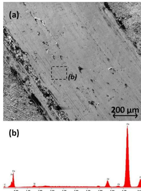
Fig. 6. (a) Characteristic SEM micrograph of the worn surface of nitrocarburised steel (A), tested in configuration (II) and (b) EDS spectrum of the area marked in (a).
