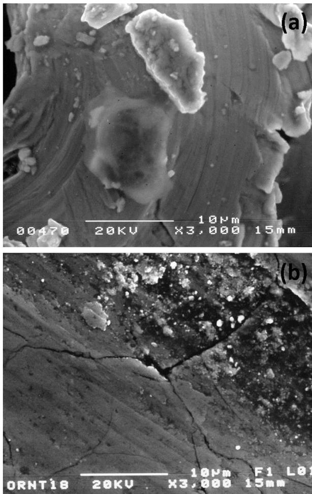
**Fig. 9.** Characteristic micrographs of the contact surfaces after steel-on-steel plane contact sliding tests: (a) Worn surface of soft-annealed steel (C) showing deformation patterns, (b) Worn surface of nitrocarburised steel (C); branched cracks appeared as a precursor of exfoliation and spalling.
