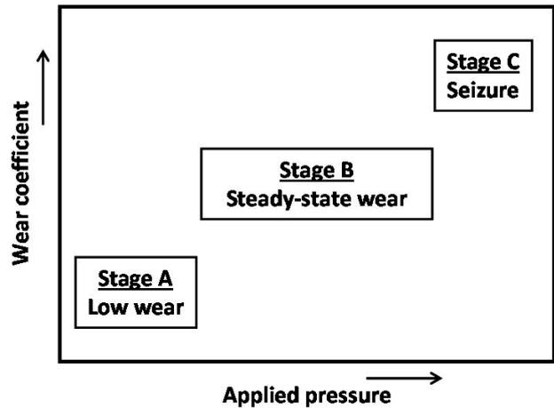
Fig. 8. Schematic of the wear coefficient evolution versus the applied pressure, for steel-on-steel plane contact sliding.
