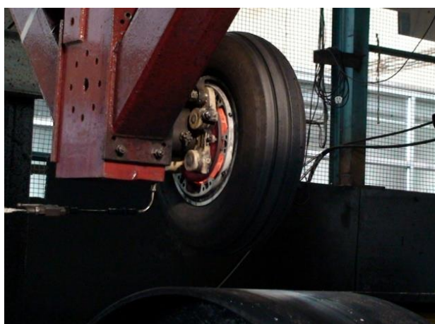
Fig. 4. Brake unit assembly in the full scale Dynamometer.
