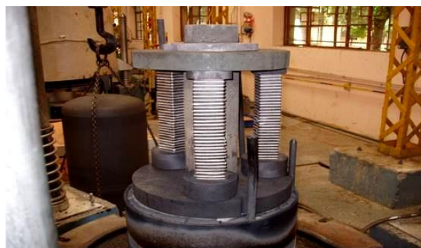
Fig. 1. Pressure sintering unit showing the alternate stacking of the back plate and green compact.
