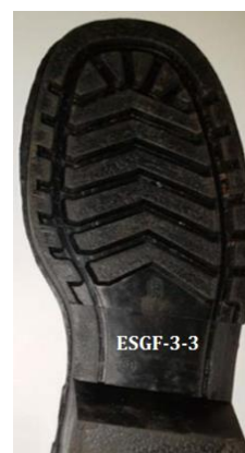
Fig. 8. Tested soles ESGF-3 (without wear).
