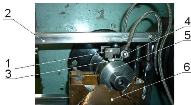
Fig. 3. The testing unit for double friction pairs: 1 – the pad screw retainment; 2 – the lever; 3 – the pad; 4 – the thermocouple-to-pad screw retainment; 5 – the rotating disc; 6 – the oil bath.
