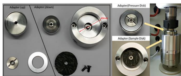
Fig. 5. Pressure disc, adapter, and friction disc sample.
