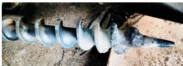
Fig. 15. Image of worn and thermal deformation screw.
