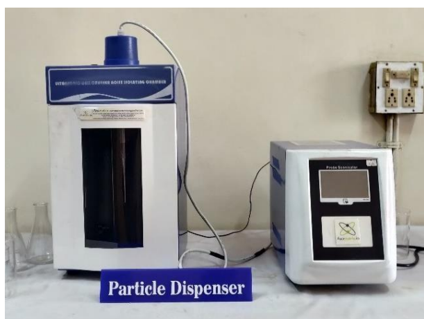
Fig. 2. Probe ultrasonicator used for particle dispersion.
