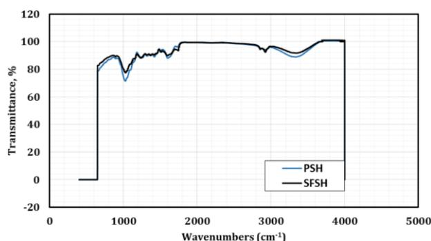
**Fig. 9.** Fourier Transform Infrared Spectroscopy FTIR for sunflower seeds and peanut seeds.
