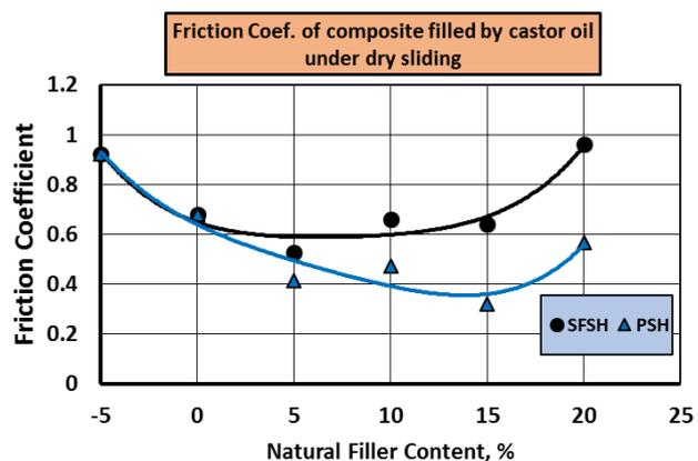
Fig. 3. Effect of natural fillers on the friction coefficient of epoxy hybrid composites filled with castor oil.
