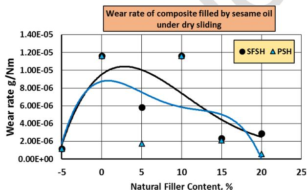
Fig. 2. Effect of natural fillers on the wear rate of epoxy hybrid composites filled with sesame oil.
