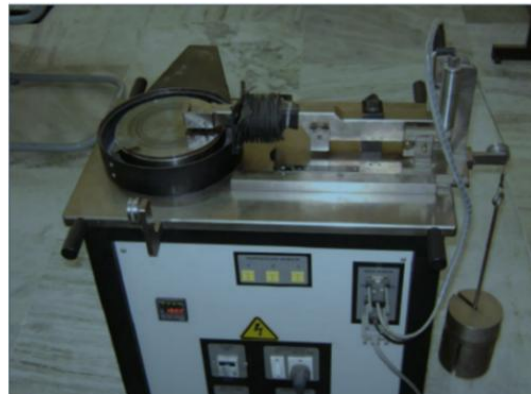
Fig 5. Pin on disk setup Test parameters: Load = 10 N to 30 N, Speed = 2 m/s to 4 m/s, Distance = 1000 - 3000 m. The wear loss was measured after each test.
