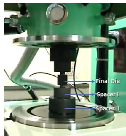
Step II. Die Placement in SPS machine
