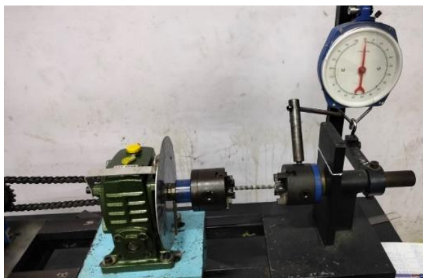
Fig. 13. Reduction gear loading in torque tests.
