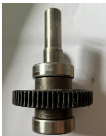
Fig. 12. Worm gear ring composite assembly.
