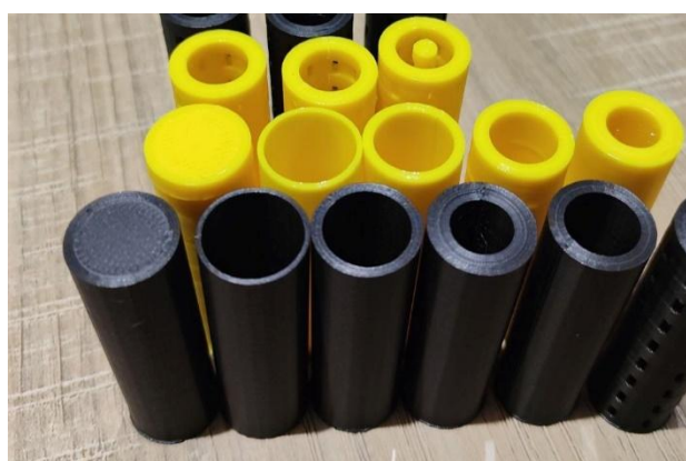
Fig. 2. shows the final appearance of PLA and CF-PLA samples prior to the epoxy casting process.
