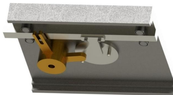
Fig. 2. Eccentric shaft and linear motion table.
