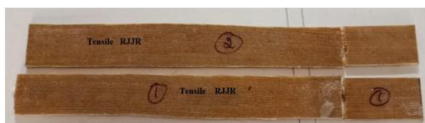
(c) Tensile fractured specimen (RJJR)
