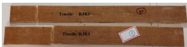
(a) Tensile fractured specimen (RJRJ)
