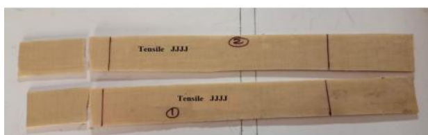
(b) Tensile fractured specimen (JJJJ)
