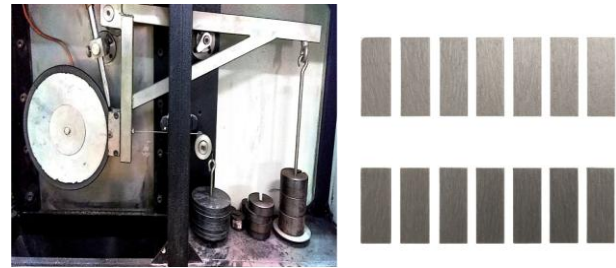
Fig. 4 Abrasive test rig and samples used for three body abrasion testing
