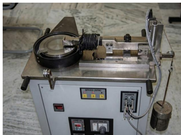
Fig. 1. Pin-on-disc tribometer employed for friction and wear experiments.
