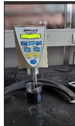
Fig. 16. Viscosity measurement for 0.1% wt. concentration of CuO based nanolubricant pre-testing.
