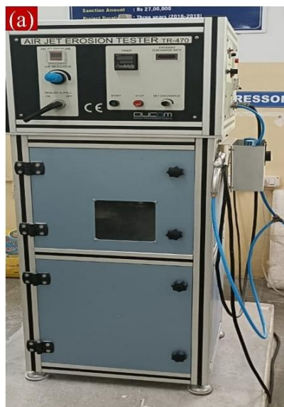
Fig. 3. Experimental set up of air jet erosion test rig.
