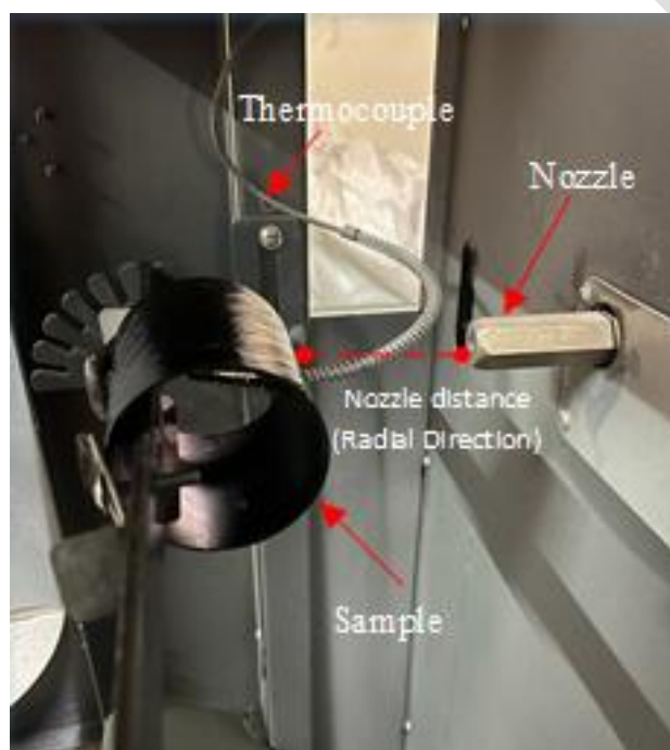
Fig. 2. Placing samples in the testing rig.
