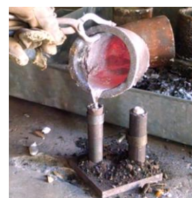
Pouring Molten MMC's in Moulds
