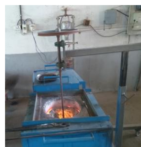
Addition of reinforcement along with stirring
